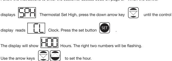
When the correct hour is displayed, press the set button
